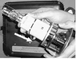
5) Reposition the lamp assembly and replace the two screws (**D**) removed previously.
