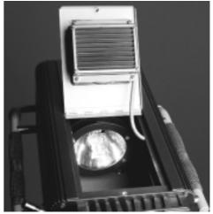
After this simple operation, you will have direct access to the lamp assembly to perform any necessary maintenance.
