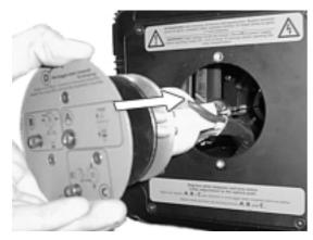
Attention: DO NOT use the projector without first undertaking the realignment of the lamp in the optical train. This ensures that no internal parts are overheated due to incorrect focusing. Refer to section 13 of this manual for instructions regarding lamp alignment.
